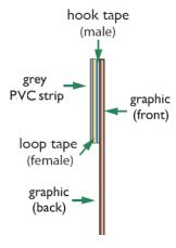
Add 0.63" (16mm) hook tape (male) to the top of the new graphic panel and apply the existing grey PVC strip.
