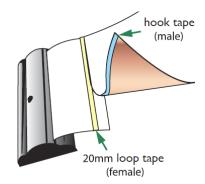
Carefully remove the existing graphic panel from the PVC tongue. Add 0.78" (20mm) hook tape (male) to the base of the new graphic panel and then place in the same position.
