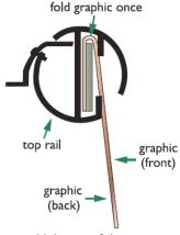
Fold the top of the new graphic backwards once and then slide into the top rail.
