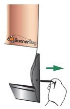
While carefully holding the graphic, remove the pin from the side of the system and gently allow the graphic to roll back into the unit.
