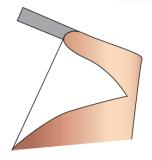
Slide the top rail off the old graphic panel and carefully remove the grey PVC strip (female loop attached) from the print.
