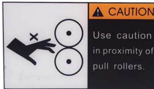
When using a large supply roll, be aware that a pinch hazard may exist between the top roller and the supply shaft. When working from the rear of the machine, be aware of the pinch point (Nip area) of the contacting rollers and exercise extreme caution to avoid injury.
